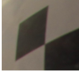
Figure 7. Example of chromatic aberration. Notice the green and magenta artifacts at the edges of the squares.
